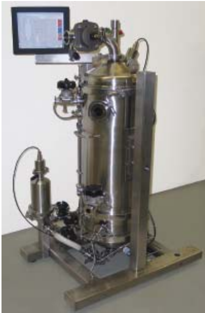
Figure 3. Representation of ATF-4 with transducers to measure flow characteristics.
